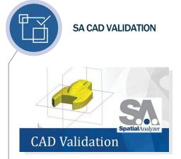
The SA CAD Validation application is a separate utility that allows you to define standalone test reference files that contain lists of CAD files and reference points for verification.
